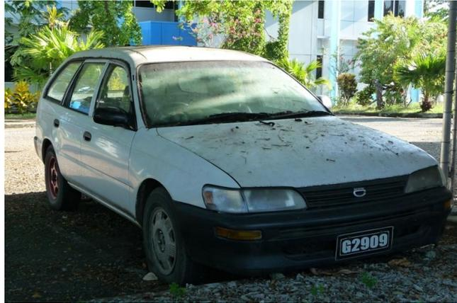
The government vehicle in this picture is typical of many that are poorly maintained in the SIG fleet. It is no longer serviceable and at the time of audit had been left in the MoFT compound to decay.
